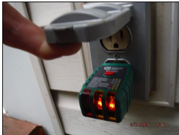
8. No GFCI (Ground Fault Circuit Interrupter)
